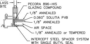
7/8" INSULATED ANNEALED/TEMPERED IMPACT GLASS WITH 0.060" PVB INTERLAYER
